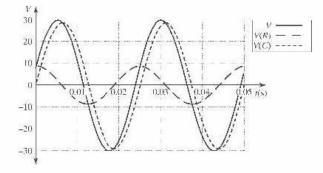
b) The different voltage are:  $v = (30.0 \text{ V}) \cos(250t - 73.3^\circ), v_R = (8.62 \text{ V}) \cos(250t), v_C = (28.7 \text{ V}) \cos(250t - 90^\circ)$ At t = 20 ms :  $v = -25.1 \text{ V}, v_R = 2.45 \text{ V}, v_C = -27.5 \text{ V}$ . Note  $v_R + v_C = v$ . c) At t = 40 ms :  $v = -22.9 \text{ V}, v_R = -7.23 \text{ V}, v_C = -15.6 \text{ V}$ . Note  $v_R + v_C = v$ . Careful with radians vs. degrees!
